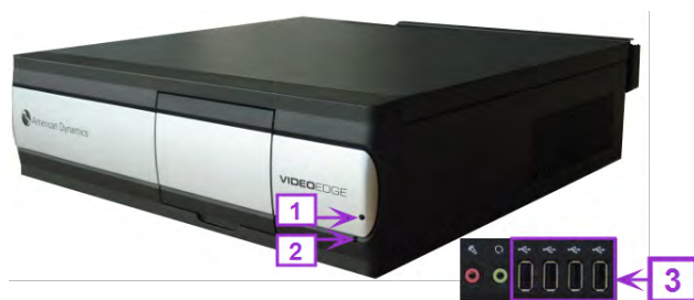
Figure 80: VideoEdge Desktop NVR front view
