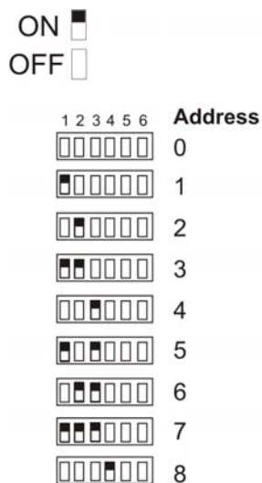
Figure 1.3 . Set DIP Switches on the 6815
